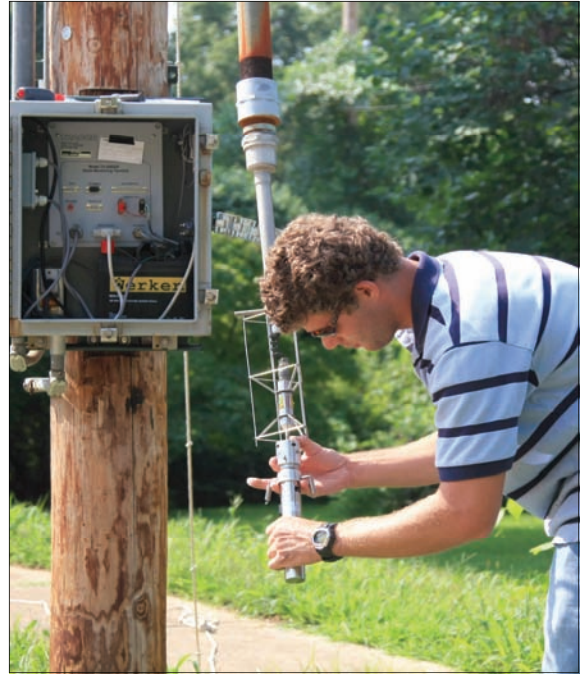
Technician attaching a pistonphone to the microphone when performing calibration. Each microphone and all computer equipment are calibrated annually.
