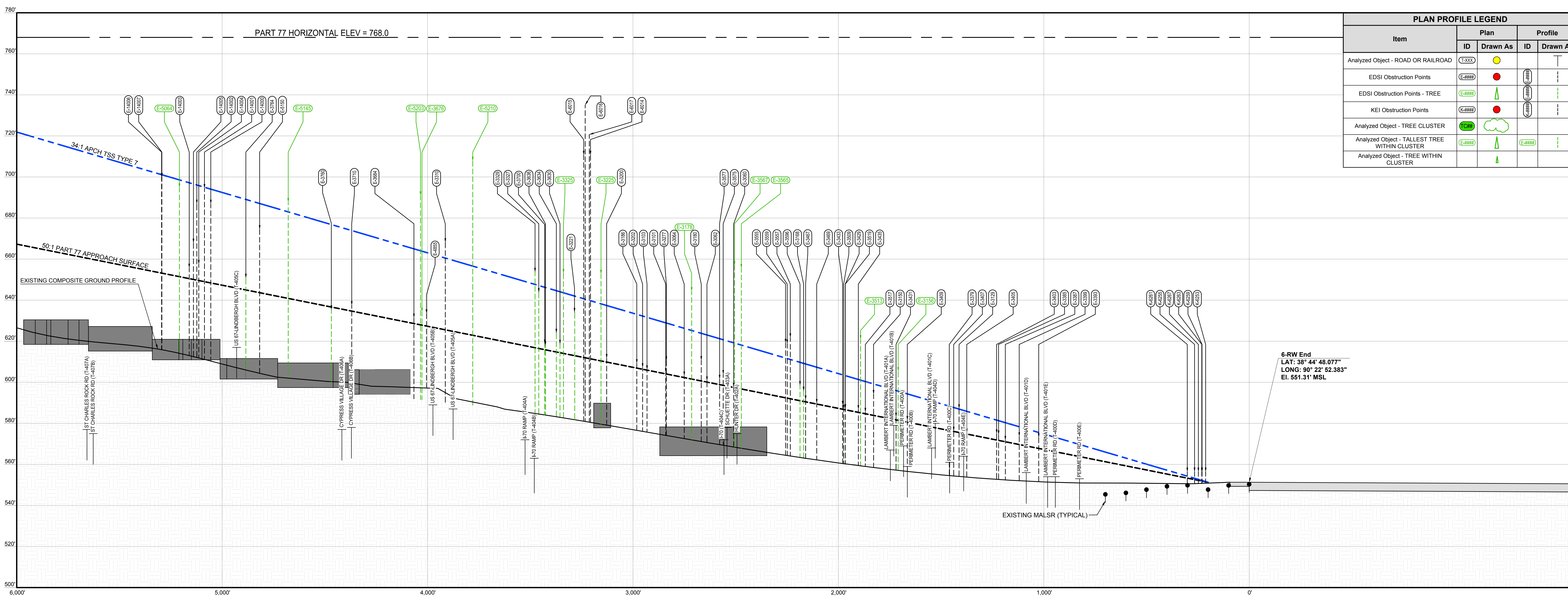
RUNWAY 6 PROFILE VIEW SCALE: 1" = 20' (VERTICAL) 1" = 200' (HORIZONTAL)
