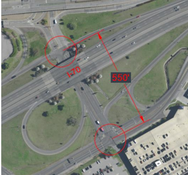
Figure 4.3-9: Insufficient Interchange Ramp Separation
