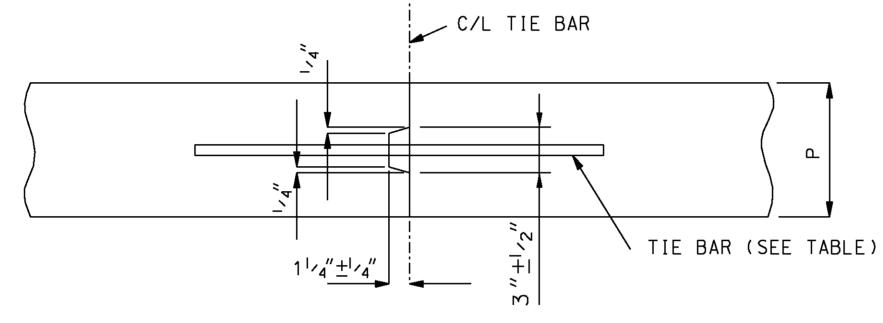
IF METAL IS USED TO FORM KEY DISCONTINUE STRIP FOR DISTANCE OF APPROXIMATELY 3" EACH SIDE OF TRANSVERSE JOINT.
