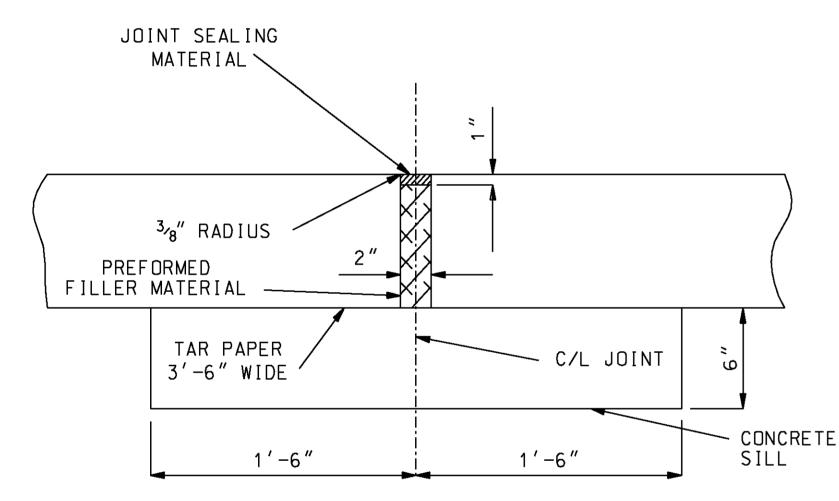
SILL SHALL EXTEND 18" BEYOND EACH EDGE OF THE PAVEMENT, AND SHALL BE CONSTRUCTED OF CONCRETE REGARDLESS OF ADJACENT BASE MATERIAL.
