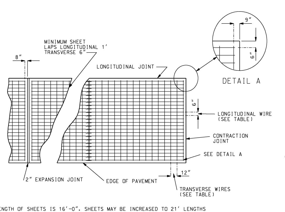
LENGTH OF SHEETS IS 16'-0". SHEETS MAY BE INCREASED TO 21' LENGTHS PROVIDED PROOF IS SUPPLIED BY THE CONTRACTOR THAT ANTICIPATED PAVING PROGRESS AND ROADWAY CURVATURE WILL PERMIT PLACEMENT
