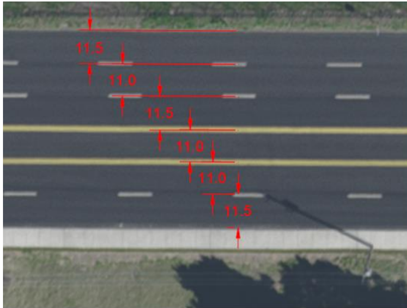
Figure 4.3-10: Airport Rd. Shoulder and Signalized Intersections Spacing Deficiencies
