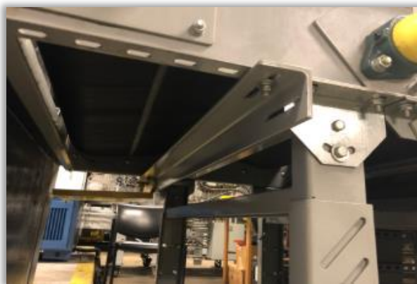
Figure 11.2-22: T2 Transport Conveyor – Belly Cover Missing
