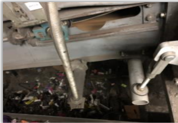
Figure 11.2-21: T2 Decline Conveyor – Safety Guard Missing
