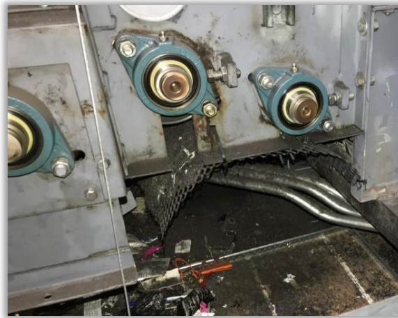
Figure 11.2-19: T2 Transport Conveyor – Missing Bearing Caps
