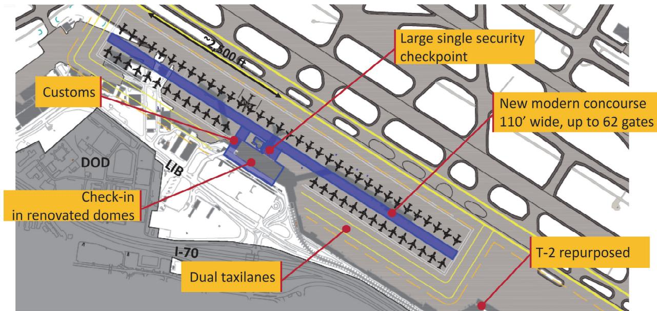
ensure that the shortlisted terminal alternatives were appropriate and that all options and suggestions had been considered. The preferred terminal alternative consists of consolidating all airlines in an efficient single terminal with a linear concourse that can accommodate up to 62 gates. The iconic domes are retained and become the centerpiece for a vastly improved customer experience.
